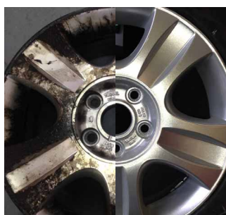
Alloy refurbishment - before and after
